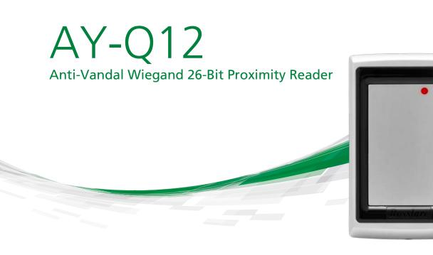
ROSSLARE'S AY-Q12 IS A UNIQUE COMBINATION OF RFID PROXIMITY READER WITHIN A METALLIC HOUSING. THIS FULLY SEALED, EPOXY POTTED UNIT PROVIDES A WEATHERPROOF AND VANDAL-RESISTANT SOLUTION FOR EXTREMELY HARSH ENVIRONMENTS. THE READER OPERATES WITH 125 KHZ PROXIMITY CARDS AND TAGS, WITH WIEGAND 26-BIT OUTPUT AND A READ RANGE OF UP TO 55 MM (2 IN.).
